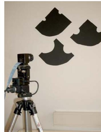
*Figure 5: a) Experimental set-up consisting of an xy-table and a stationary CMOS camera, to evaluate the localization accuracy on real images. b) Image of the shifted target, captured by the CMOS camera.*
