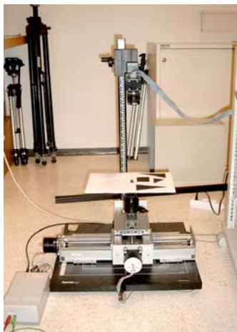
Figure 5: a) Experimental set-up consisting of an xy-table and a stationary CMOS camera, to evaluate the localization accuracy on real images. b) Image of the shifted target, captured by the CMOS camera.
