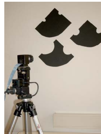
Figure 6: Experimental set-up to determine the runtime performance of the subpixel corner detector
